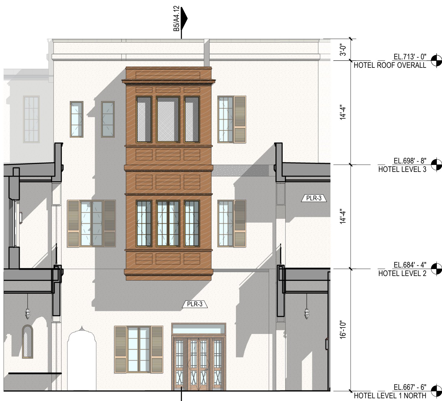
1/8" = 1'-0" COURTYARD 2 - WEST ELEVATION | B3
