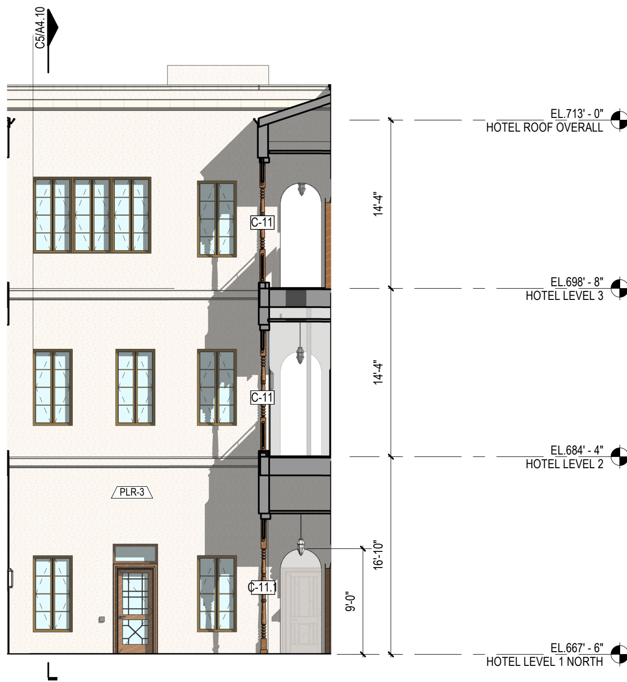
1/8" = 1'-0" COURTYARD 03 - NORTH ELEVATION | C2
