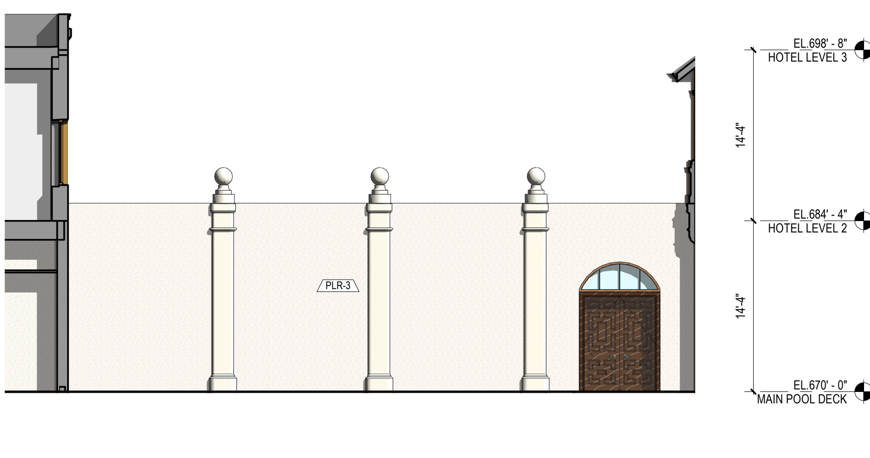
1/8" = 1'-0" POOL DECK - EAST ELEVATION | A4
