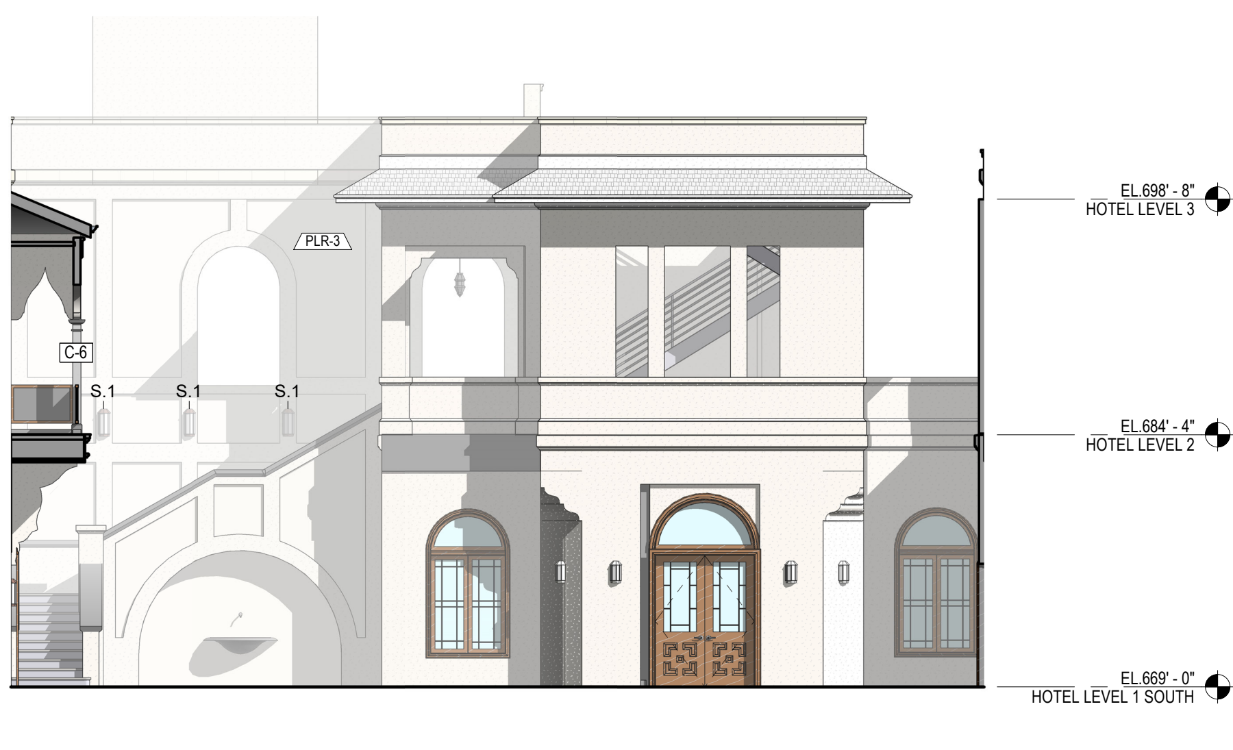
1/8" = 1'-0" GREENHOUSE COURTYARD ENTRY - ELEVATION | D4
