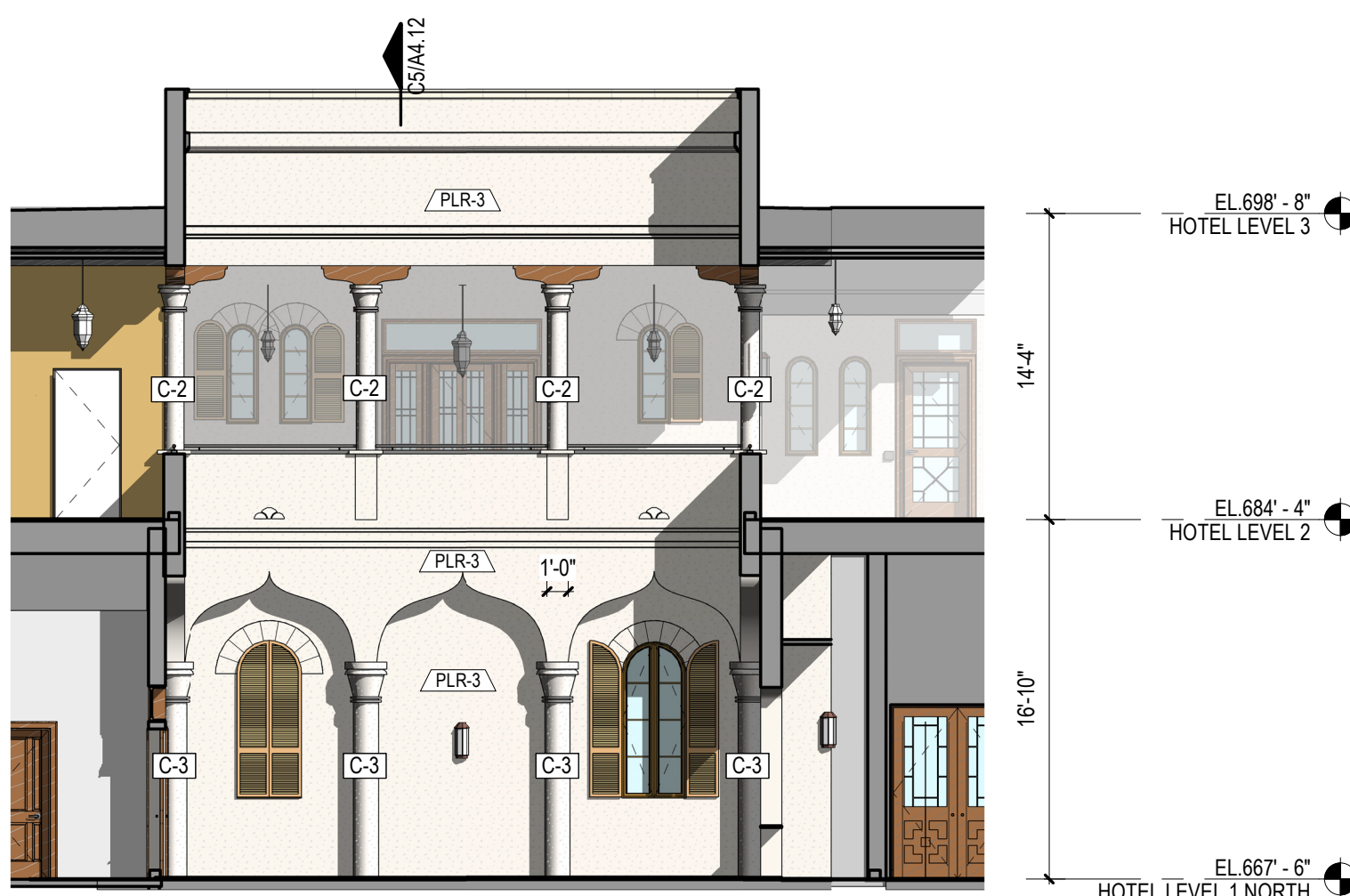
1/8" = 1'-0" EVENT COURTYARD - EAST ELEVATION | B2
