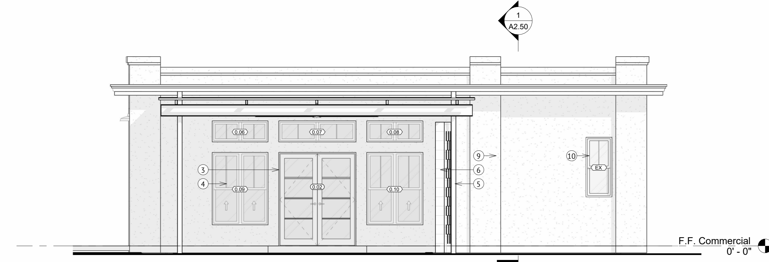
3 COMMERCIAL ELEVATION - SIDE at PARK SCALE: 1/4" = 1'-0"
