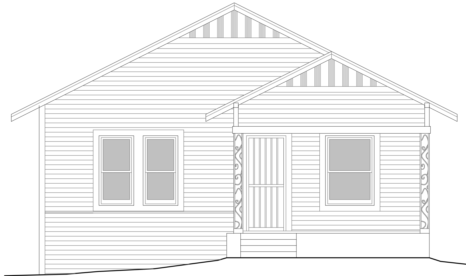
West 01 EXTERIOR ELEVATION SCALE: 1/4"=1'-0" WEST
