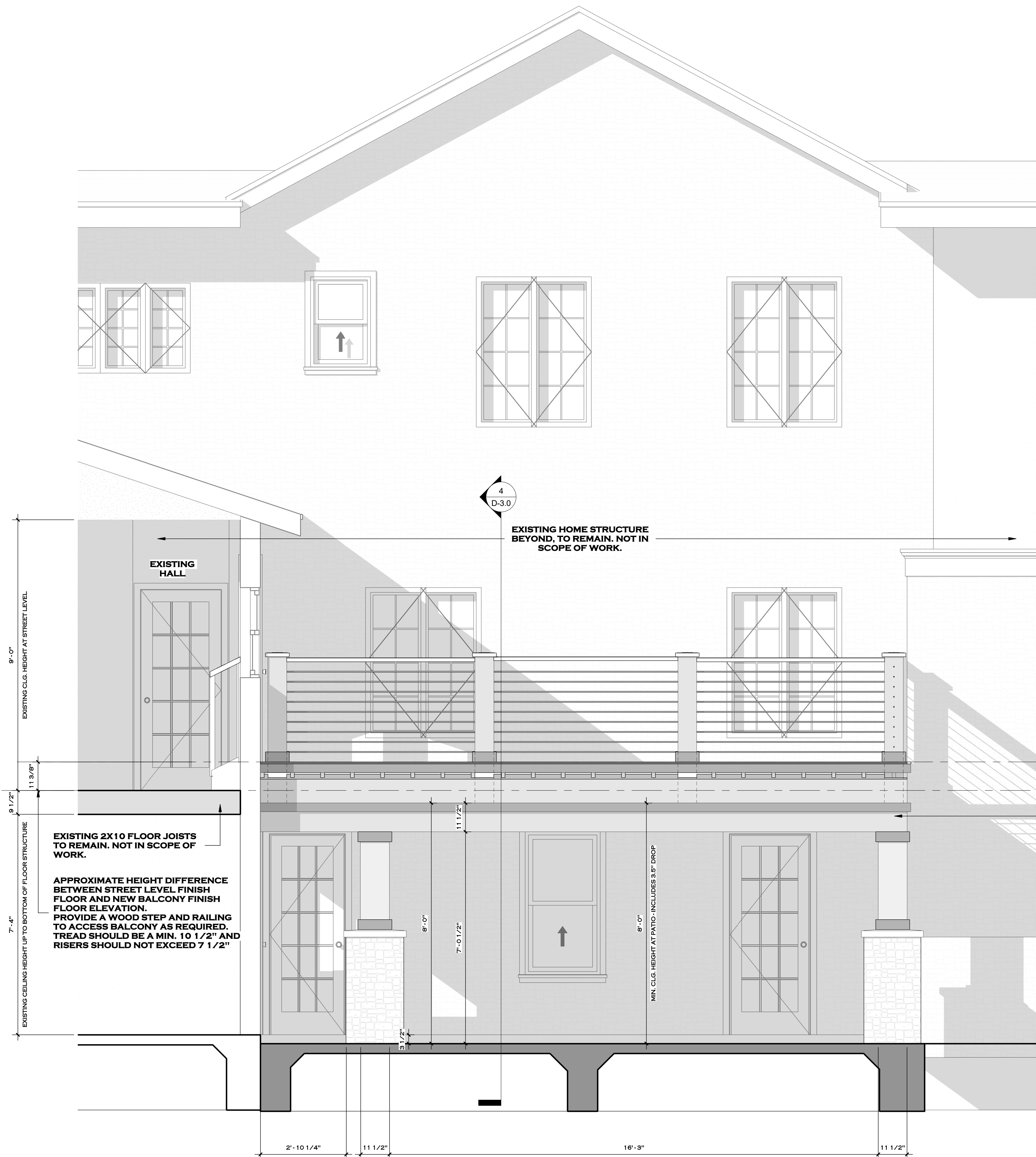
4 PATIO-BALCONY ADDITION - FRONT ELEVATION 1/2" = 1'-0"
