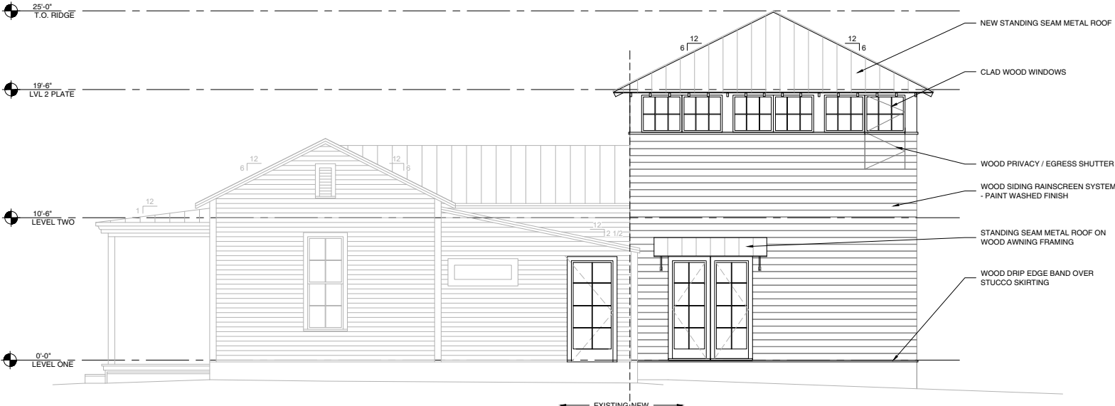
EXTERIOR ELEVATION - EAST 04 1/4" = 1'-0"
