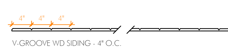
V-GROOVE WD SIDING - 4" O.C.
