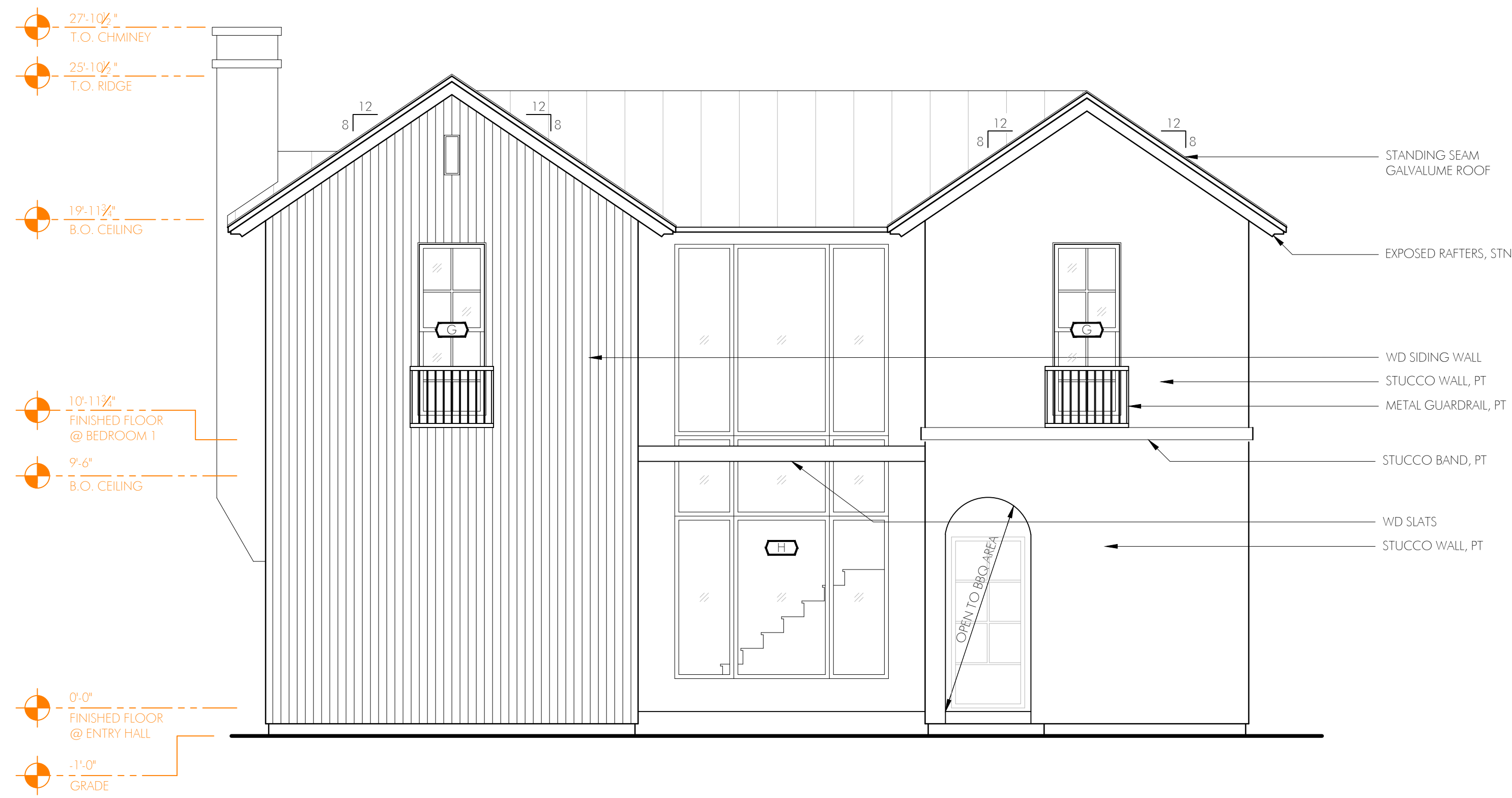
1 ELEVATION: LOOKING NORTH SCALE: 1/4" = 1'-0"
