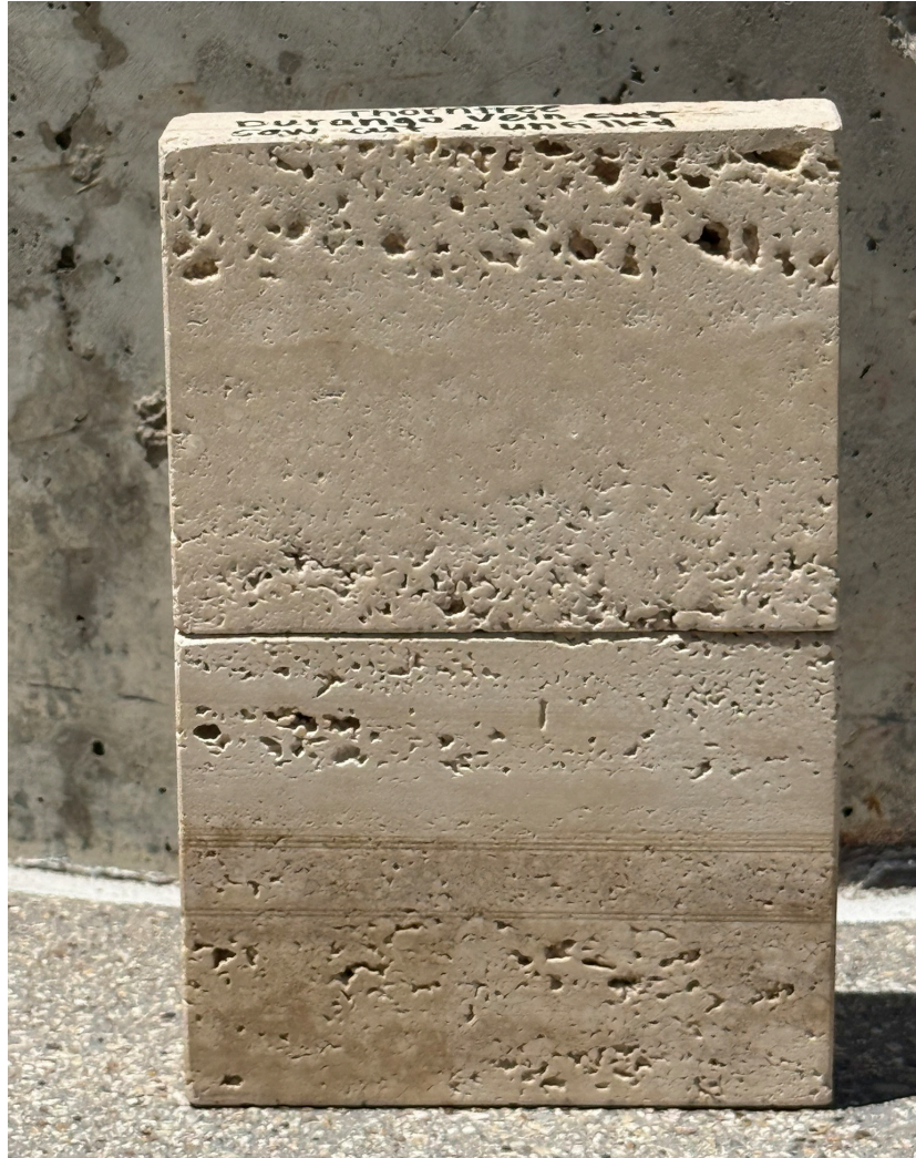
ESC-01 | STONE FINISH/COLOR: DURANGO VEIN-CUT TRAVERTINE ROUGH TEXTURED + UNFILLED SLAB (MA1177) PATTERN AND SIZE: STACKED - (REF. TO ENLARGED ELEVATIONS) NOTES: REF. TO A5.000 FOR ADDITIONAL NOTES
