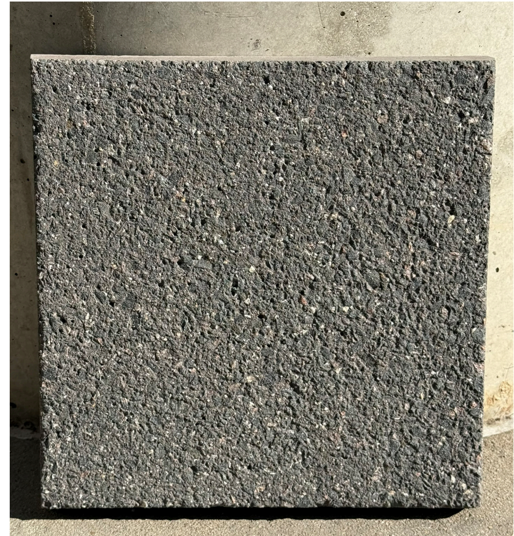
APC-03B | DARK PRE-CAST PANEL COLOR: MATCH SAMPLE #GPH-2461 FINISH: MULTI FINISH, SAND BLASTED DEEP NOTES: REF. TO A5.000 FOR ADDITIONAL NOTES
