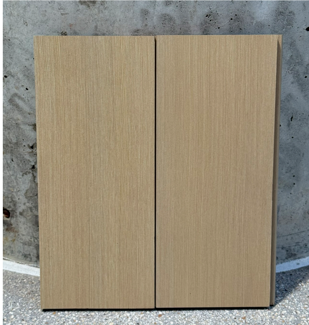
WD-01 | EXTERIOR WOOD SPECIES: THERMAL HEMLOCK TEXTURE: SMOOTH FINISH: SONOMA GRADE: CLEAR VG PROFILE: TONGUE AND GROOVE NOTES: REF. TO A5.000 FOR ADDITIONAL NOTES
