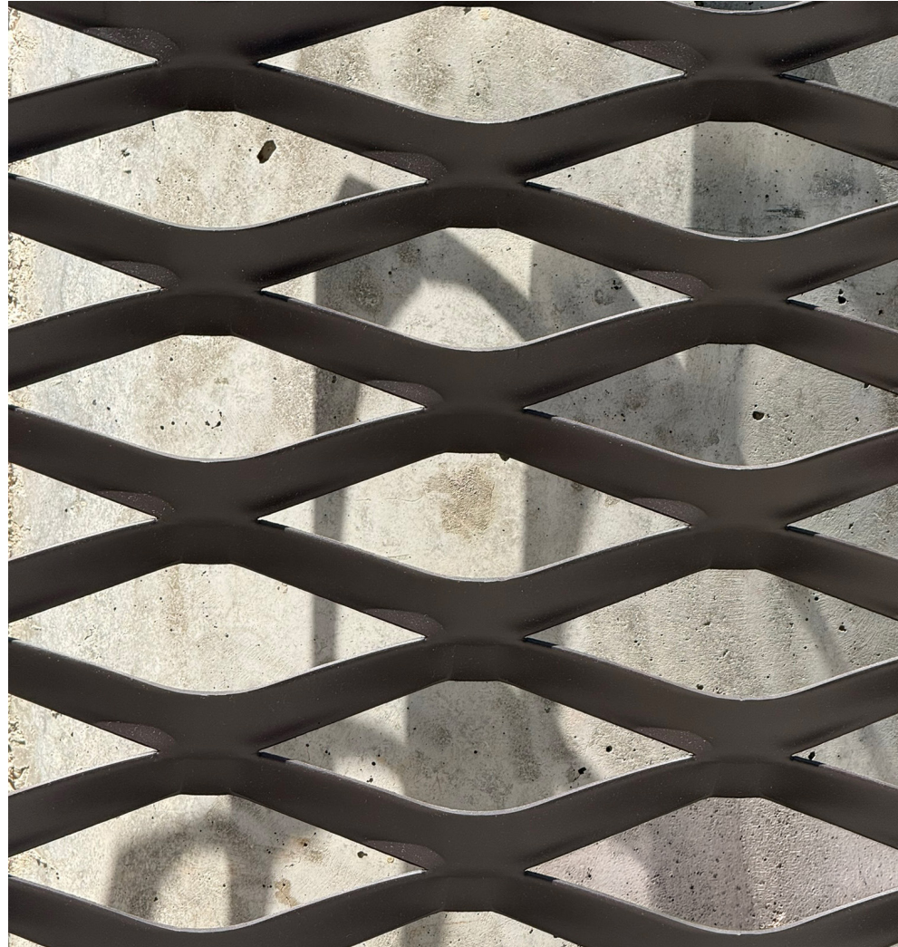
EMM-01 | EXPANDED METAL MESH SHORT WAY DIAMOND: 3.05" LONG WAY DIAMOND: 8" VISUAL OPEN AREA: 40% MECHANICAL OPEN AREA: 80% FINISH: MATCH COLOR TO AMF-03 NOTES: REF. TO A5.000 FOR ADDITIONAL NOTES
