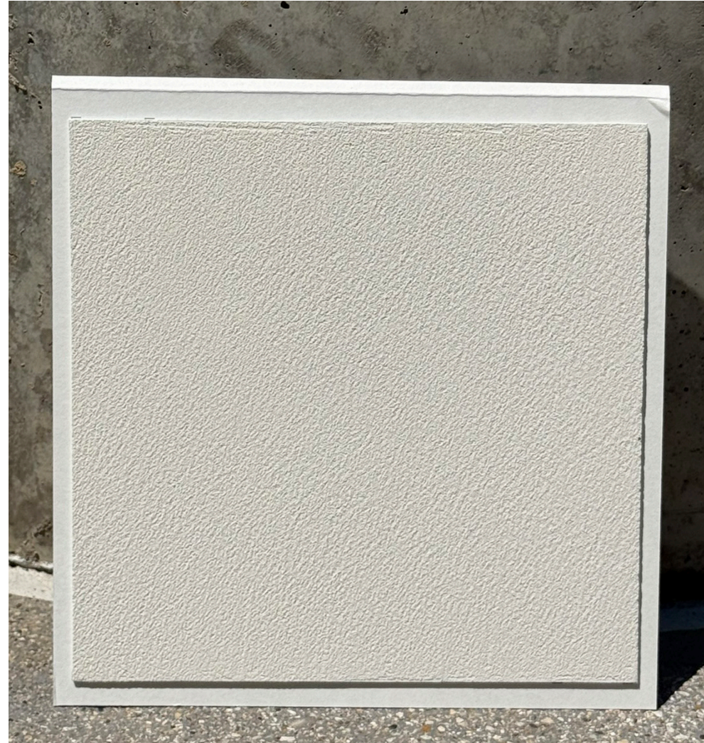
DEFS-01 | LIGHT SOFFIT COLOR: SW9166 DRIFT OF MIST TEXTURE: STOLIT FREEFORM COATING: STOCOLOR ACRYL PLUS (MATTE SHEEN) - TINTED TO SW9166 NOTES: REF. TO A5.000 FOR ADDITIONAL NOTES
