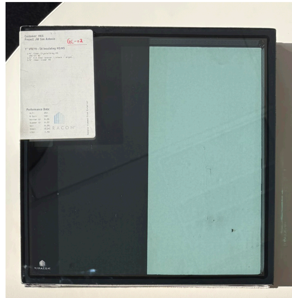
GL-02 | IGU - VISION - TOWER "DARK" VIRACON 1" VRE-19-54 INSULATING HS/HS EXTERIOR GLASS PLY: 1/4" CRYSTALGRAY COATING: VRE-54 ON #2 SURFACE SPACE: 1/2" VTS™ BLACK SPACER - ARGON FILLED SILICONE: BLACK INTERIOR GLASS PLY: 1/4" CLEAR NOTES: REF. TO A5.000 FOR ADDITIONAL NOTES
