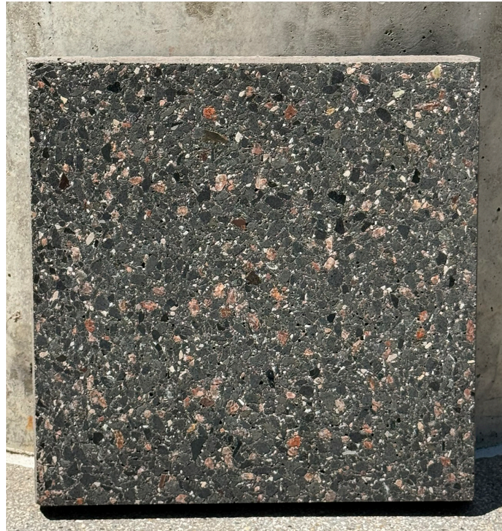
APC-03A | DARK PRE-CAST PANEL COLOR: MATCH SAMPLE #GPH-2461 FINISH: MULTI FINISH, ACID ETCHED, MEDIUM. POLISHED. NOTES: REF. TO A5.000 FOR ADDITIONAL NOTES
