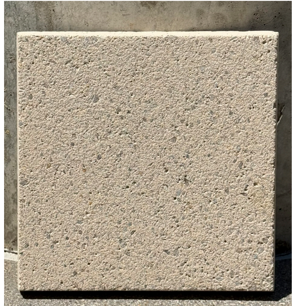
APC-02B | LIGHT PRE-CAST PANEL COLOR: MATCH SAMPLE #GPH-2469 FINISH: SAND BLASTED MEDIUM W/ ACID ETCHED AFTER. NOTES: REF. TO A5.000 FOR ADDITIONAL NOTES
