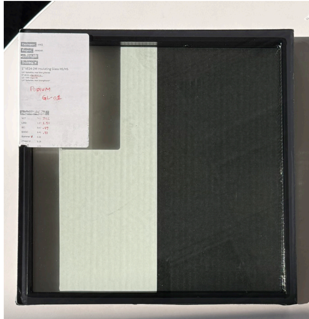
GL-01 | IGU - VISION - PODIUM - L1 / L2 VIRACON 1" VE24 - 2M INSULATING HS/HS EXTERIOR GLASS PLY: 1/4" OPTIWHITE COATING: VE-2M ON #2 SURFACE SPACE: 1/2" VTS™ BLACK SPACER - ARGON FILLED SILICONE: BLACK INTERIOR GLASS PLY: 1/4" OPTIWHITE NOTES: REF. TO A5.000 FOR ADDITIONAL NOTES
