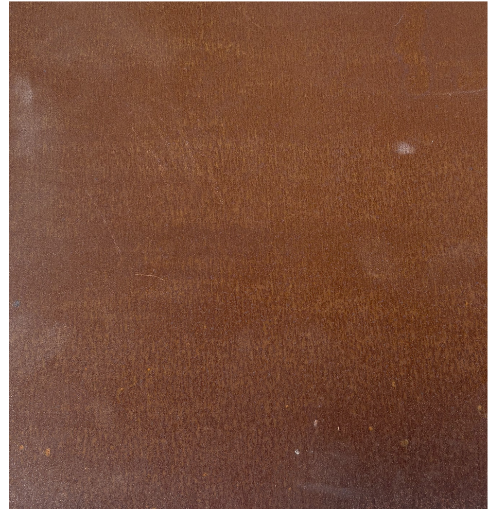
M.09 | WEATHERED STEEL COLOR: WEATHERED FINISH - PRIMED AND PAINTED FINISH: AUTOMOTIVE SEALER TO BE APPLIED AFTER OXIDIZATION PERIOD.
