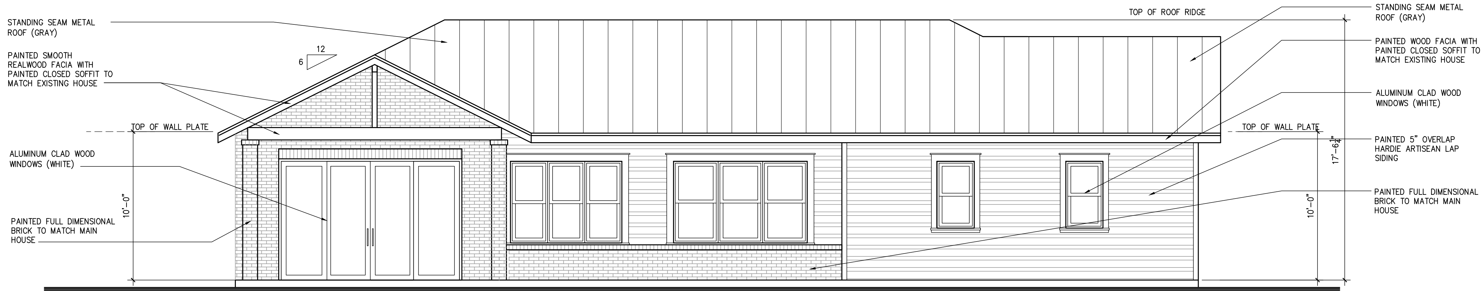
1 EAST (FRONT) ELEVATION SCALE: 1/4"=1'-0"
