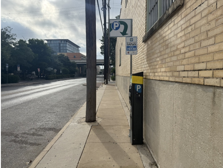
Figure 4. Obstructions in sidewalk create pinch points as sidewalk narrows to 3'10" width.
